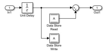
Simulink Design Verifier inserts corresponding Data Store Write blocks with inports into the extracted model.
